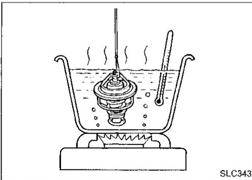
2. Check valve opening temperature and maximum valve lift.
