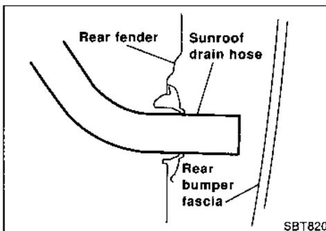
1. Remove headlining to access drain hose connections. (Refer to "ROOF TRIM", BT-29, for detail.)
